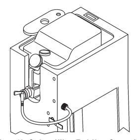
Figure 18. On-board Water Tank Hose Connection
